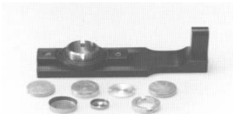
Figure. 3.13: Sample holder with brass inserts and small and large cups.
